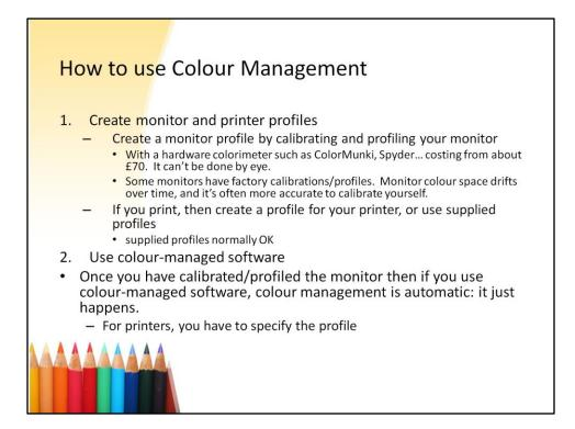
Windows control panel colour management (and I believe the same function in the Mac) contains a tool to calibrate by eye. This is better than nothing. But only just. You can adjust the tone curve (contrast) by eye approximately, but you can't accurately adjust white point by eye, and you can't measure colour space by eye.
